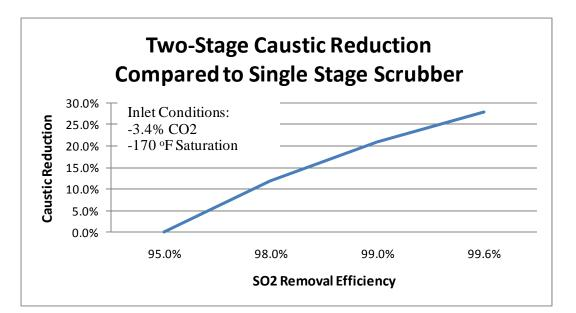
Figure 5: 2-stage reduction in caustic consumption compared to single stage scrubber.
