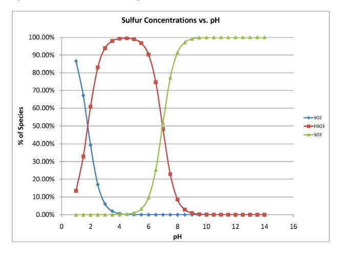
Figure 4: Sulfur concentrations versus pH.
